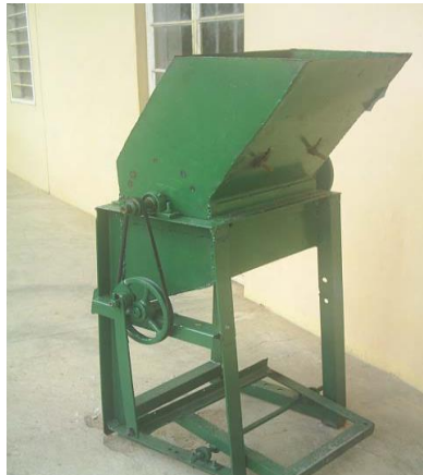
Figure 11: Display of the Treadle Operated Abrasive-Cylinder for Threshing of Cowpea
