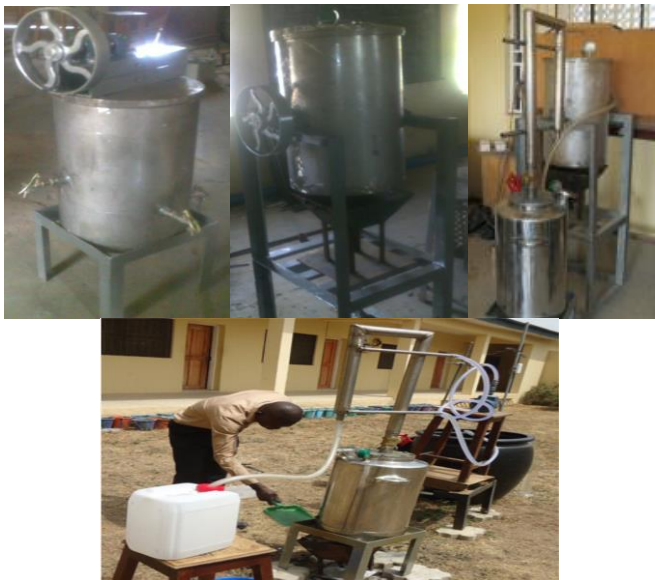
Figure 20: The views of the Fermenter Machine and Biofuel-Reflux Column Distillation Assembly.
