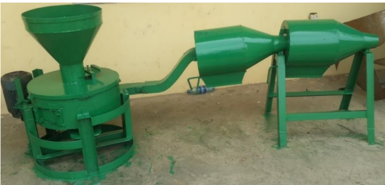
Figure 13: Pictorial View of the Fabricated Melon Shelling and Cleaning Machine
