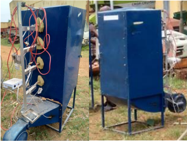
Figure 7. Photographic View of a Locust Bean Cabinet Dryer
