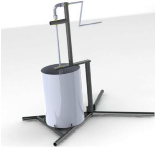
Figure 9b: Modified Version of the Milled Shea Nut Mixer with Camille George Team
