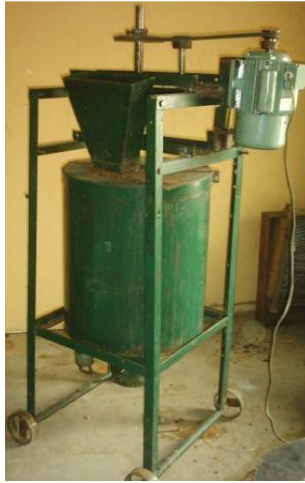
Figure 5. Photographic View of a Locust Bean Depulping Machine
