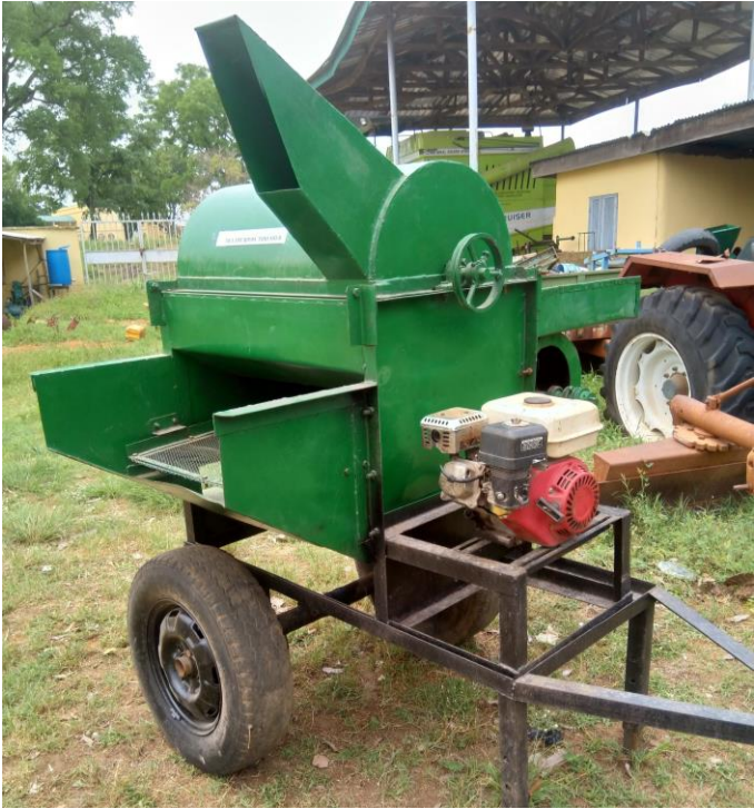
Figure 4. Photographic View of a Locust Bean Decorticating Machine
