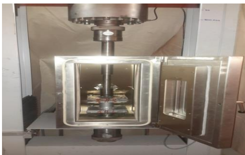
Figure 17: Display of Biomass Densification Rig inside the Heating Apparatus on the Universal Testing Machine
