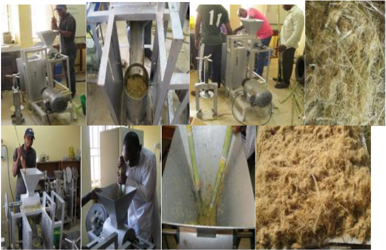
Figure 19: The views and the arrangement of the sugarcane juice extractor.
