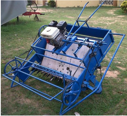
Figure 12: View of a Guided Horizontal Conveyor Rice Harvester showing the Slider-crank and other Transmission Parts
