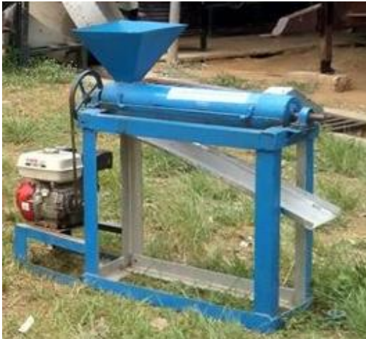
Figure 6. Photographic View of a Locust Bean Dehulling Machine
