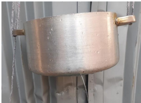
Figure 5 Leaking aluminium pot
